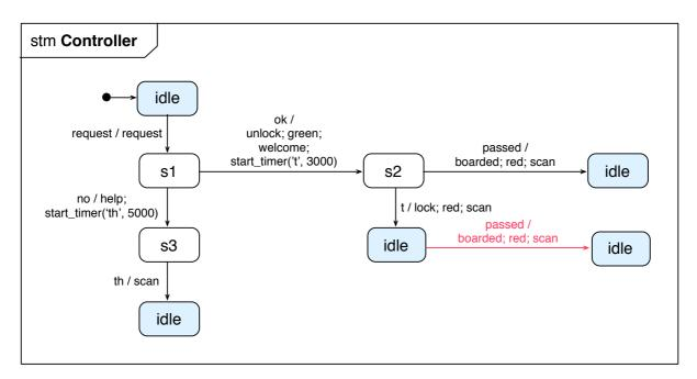
The transition (here marked in red) goes from state idle to idle (hence a self-transition) and registers the passenger with the backend. It could also be specified as an internal transition of state idle.
