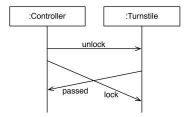
This means that the controller times out and wants to lock the turnstile again, but just after it sent the message lock, the passenger goes through and boards the airplane and the turnstile sends passed.
