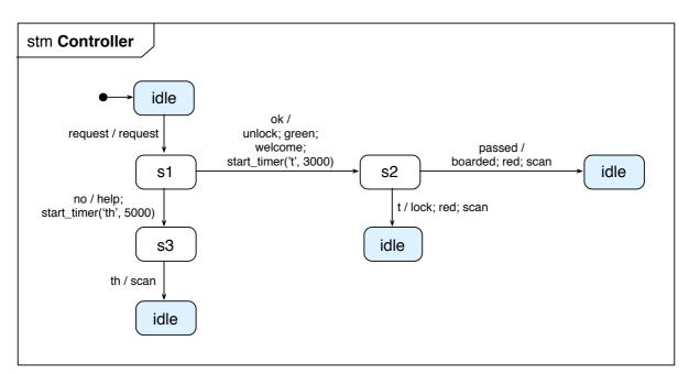
We can solve the problem by extending the state machine with a new transition:
