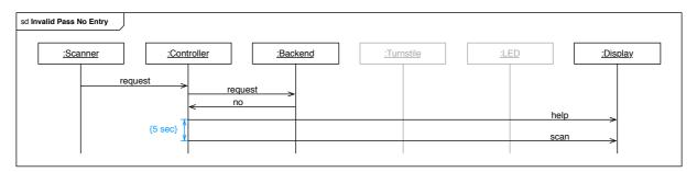
The last diagram also specifies a timing constraint (in blue) to separate the help message from the scan message for the next passenger.
